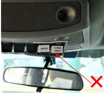
Not Acceptable – Not Permanently Label
